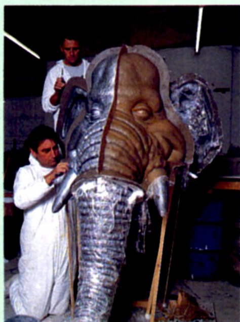
Pulling a mold off a woolly mammoth sculpt, to fabricate the design in foam rubber.
